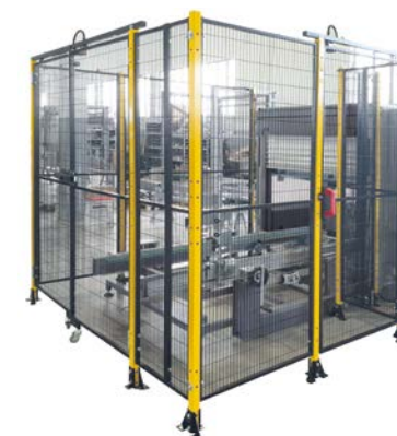
Fig. 11 Perimetral safety protections CAR
